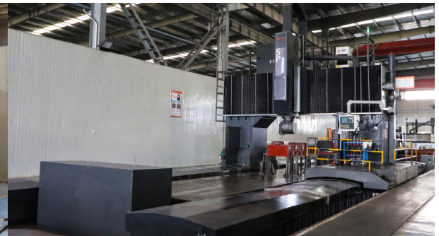
SP3212 with Nicola Correa automatic universal milling head
